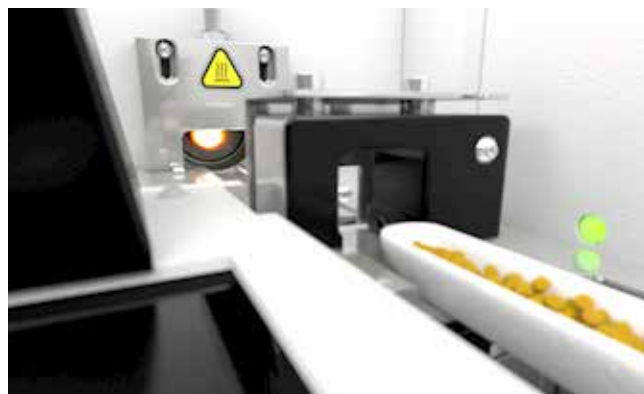
High temperature ceramics (HTC technology) for manual and automated catalyst-free combustion at up to 1300 °C
